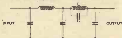
Fig. 2. The artifice of tuning one of the smoothing chokes to resonate at the predominant hum frequency does not always work out satisfactorily in practice.
